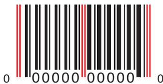
UPC-A barcodes have 12 numeric digits, and always have the slightly longer bars indicated here in red at each end and the middle. They often have the beginning and end human readable digits in a slightly smaller font, slightly beyond the bars at each end.
