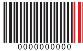
Code 128 barcodes can be any length. The human readable digits below the code are optional. The best way to recognise a Code 128 is by looking at the end bars, indicated above in red. These are identical for every Code 128 barcode.
