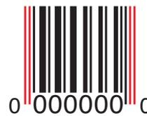
UPC-E barcodes have 8 numeric digits, and always have the slightly longer bars indicated here in red at each end. They often have the beginning and end human readable digits in a slightly smaller font, slightly beyond the bars at each end.
