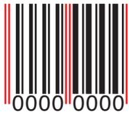
EAN 8 barcodes are 8 digits in length. They always have the slightly longer bars as indicated above in red, at either ends and the middle.
